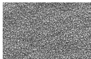
Ultra Low Profile Copper (Treated surface) x 3,000
