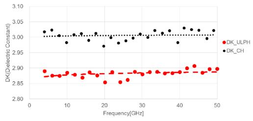
NF-30 is supplied with ULP copper foil, an Ultra-Low Profile copper foil due to its superior insertion loss at 77 GHz. The slightly lower Design DK is easily adjusted in any CAD program.
